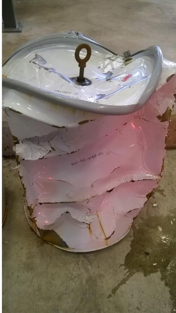
**Figure 3: Test Sample WC-HC-NDF-01 after Hyperbaric Testing**
