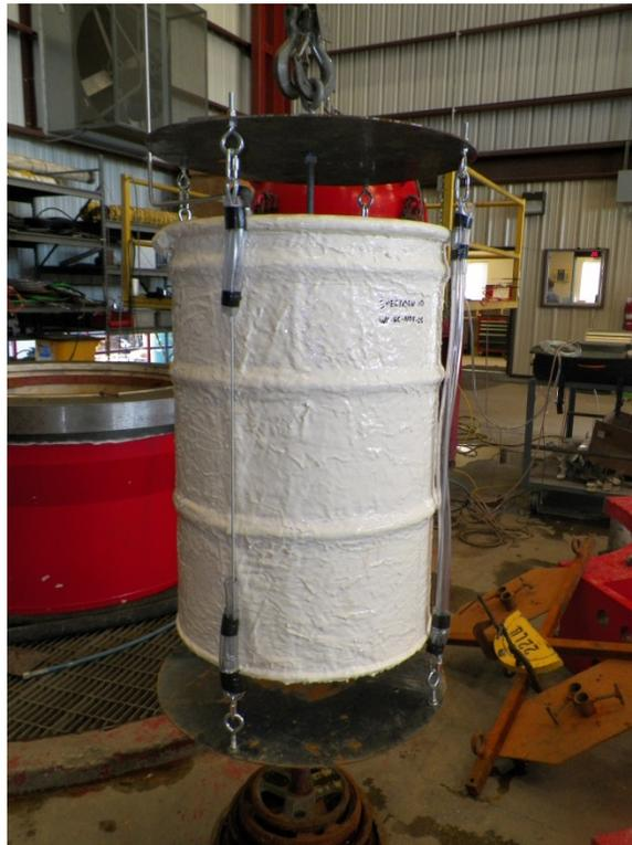
**Figure 2: Sample Mounted Inside Test Fixture**
