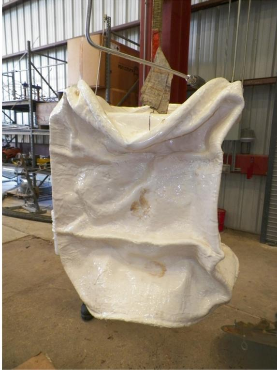
**Figure 6: Test Sample WC-HC-NDF-06 after Hyperbaric Testing**
