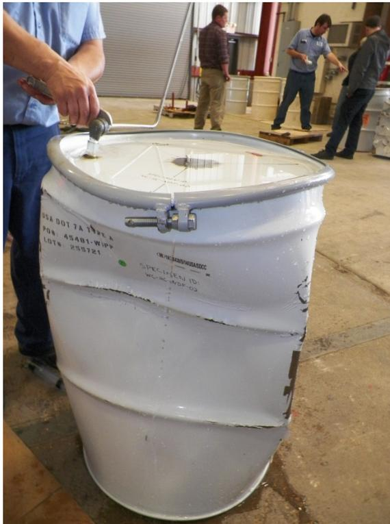
**Figure 5: Test Sample WC-HC-NDF-02 after Hyperbaric Testing**
