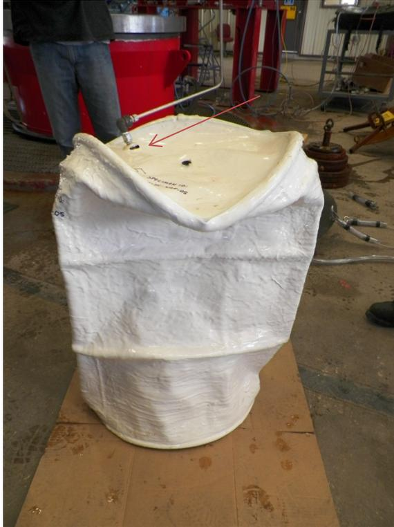
**Figure 4: Failure at Bung Location for Test Sample WC-HC-NDF-05**
